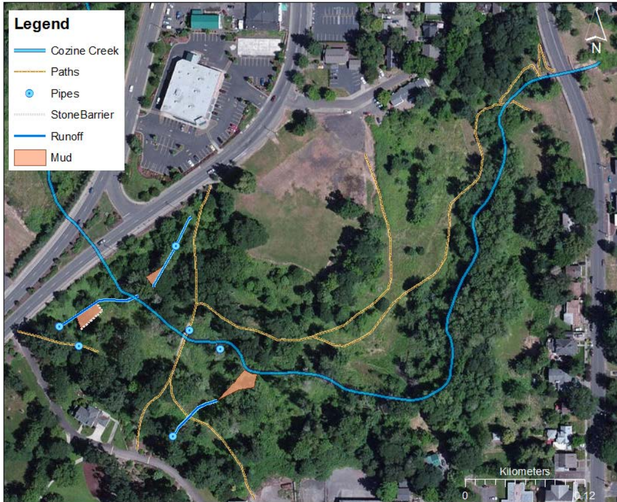
Figure 5.4 Map indicating location of stormwater pipes, the paths of their runoff, and resulting accumulations of mud
