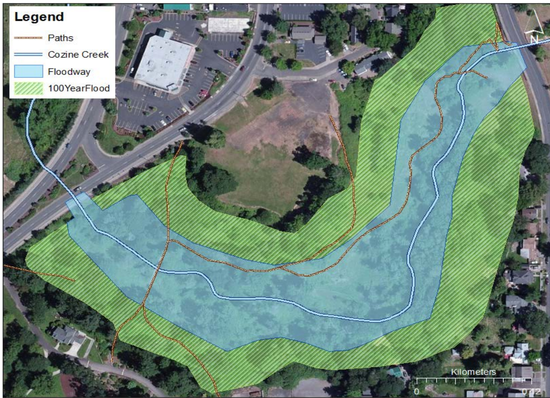
Figure 3.1 Floodway and one hundred year flood zone in Cozine Creek (Map by Rachel Blanco 2017).
